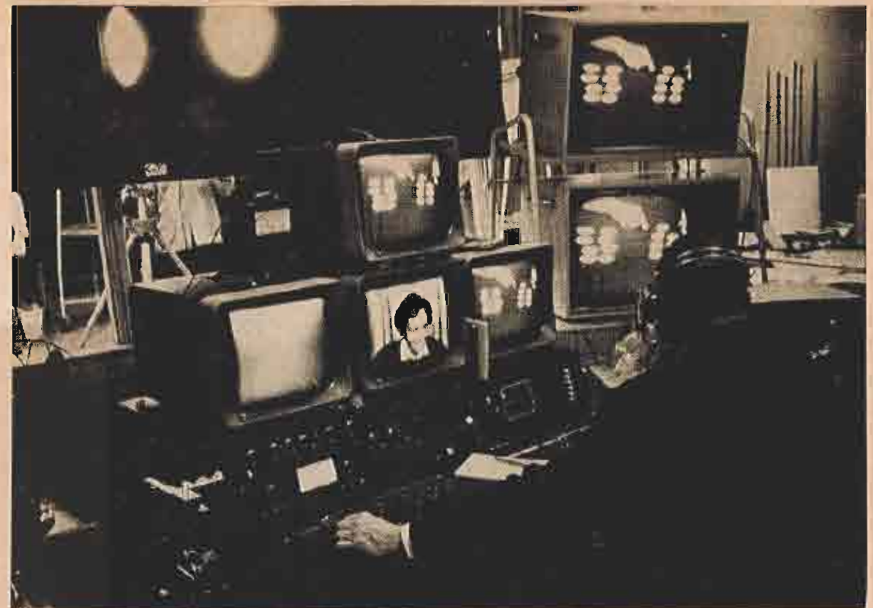
The CCTV control room at an elementary school in Chicago. A lesson in arithmetic is being televised by two cameras. The programme controller switches from one camera to the other as the lesson progresses.
