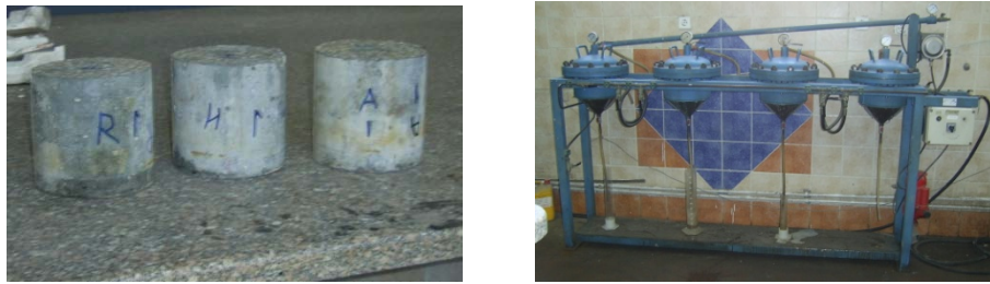
(a) Specimens (½ standard cylinders) (b) Testing apparatus Fig. 3: Specimens and apparatus used in the comparative permeability tests
