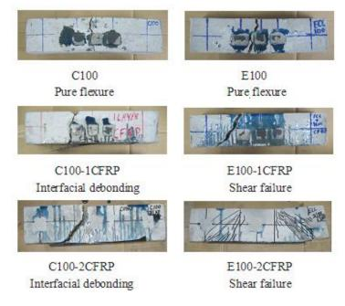
Fig. 6: Failure Patterns for the Tested Specimens
