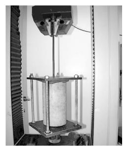
Fig. 3: Testing bond strength
