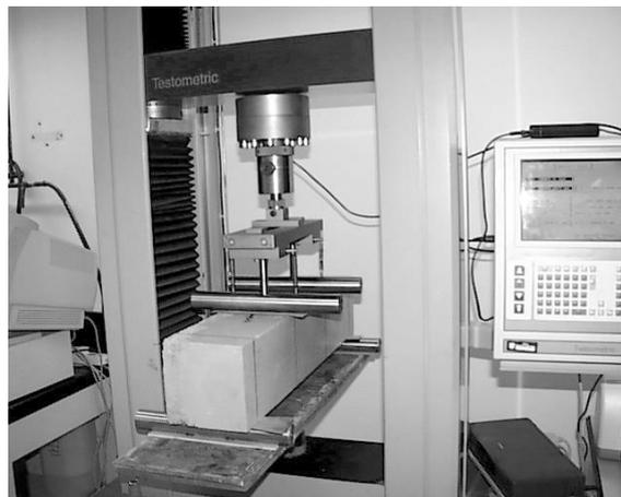
**Fig. 2: Flexural testing of beams**
