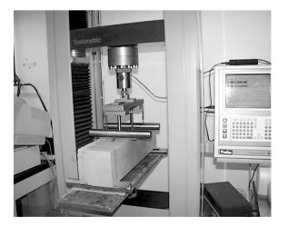
Fig. 2: Flexural testing of beams
