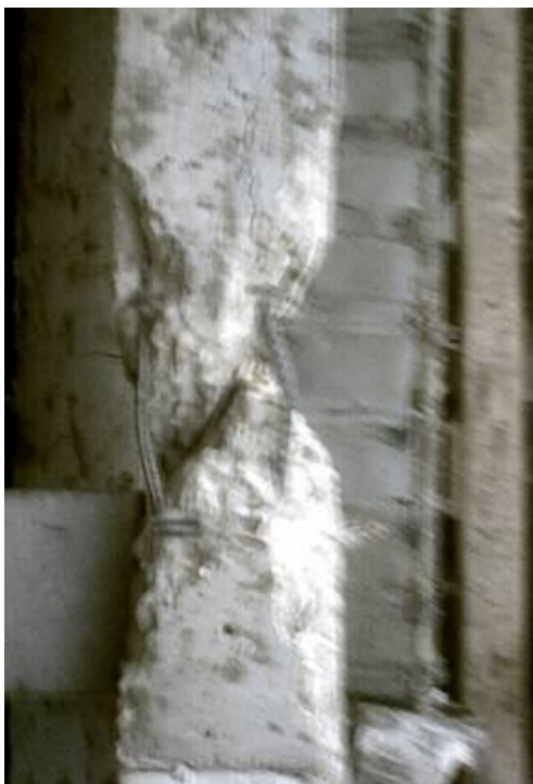
Fig.8: Failure mode shape For un-strengthened columns.
