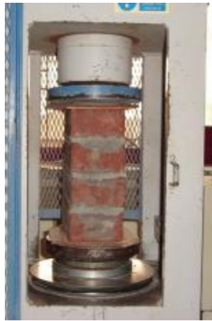
Fig. 2: Testing of Masonry Prism.
