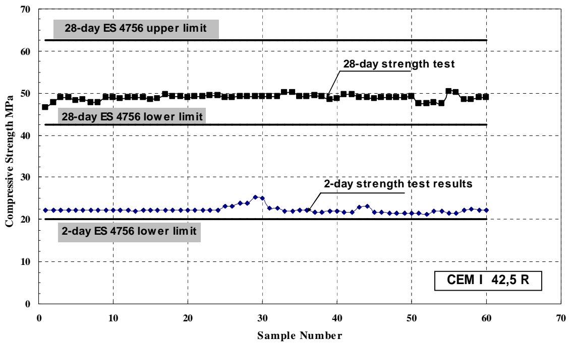
Fig. 8: 2 and 28 Day Compressive Strength for CEM I 42,5 R
