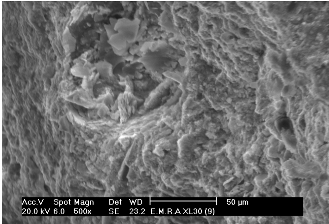
Fig. 10: SEM of Blended Cement Pastes Containing 70% 30% WCS Cured at 28 Days and Fired at 500oC for 3 Hours.
