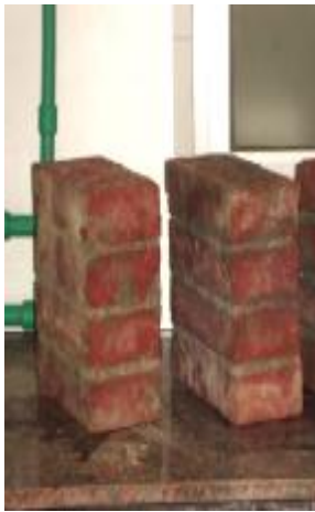
Fig. 2: Testing of Masonry Prism.
