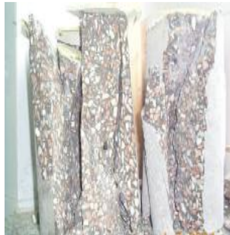
Fig. 3: Failure Mode of High Strength Concrete Cylinder.
